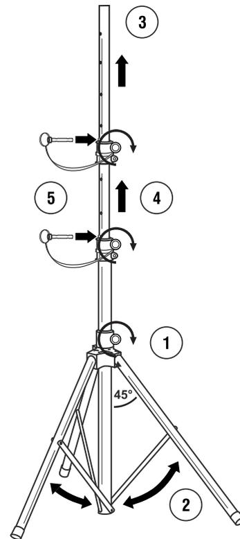
**Pull out the legs** – Loosen the safety screw (1) of the legs. Pull out the legs (2). Lock this position with the safety screw.
