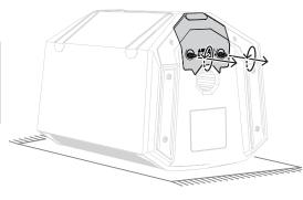
Gently but firmly pull on the battery pack by the finger pull located on the back of the battery door.
