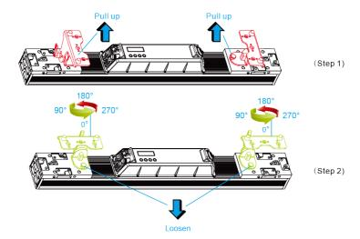
Use a hexagon wrench to rotate the locking positioning system clockwise to fasten the fixtures.
