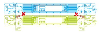
The adaptable bracket system can be rotated by pulling the locking pin. After bringing the bracket system in the right direction, make sure to fasten the locking pin.
