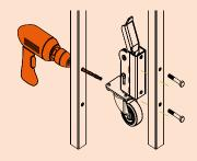
Drill two holes here and attach the wheel with 2 bolts.
